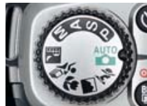
Exposure mode dial For simple control of F65 exposure modes.
